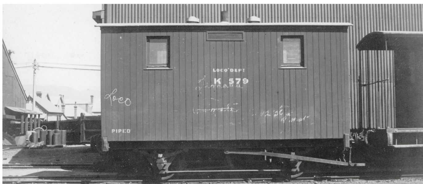
Below: K 579 at Christchurch in 1906 illustrating the opposite side to that of K578. One of the new sleeping vans built to BP1873, plan K2, this one on an ex D&PCR underframe built by Bristol Car & Waggon Co in 1872. This photo was taken by Ernest Arundel, an Australian seaman / Railway enthusiast, who visited NZ several times during 1906-8. E. Arundel, John Agnew Collection
